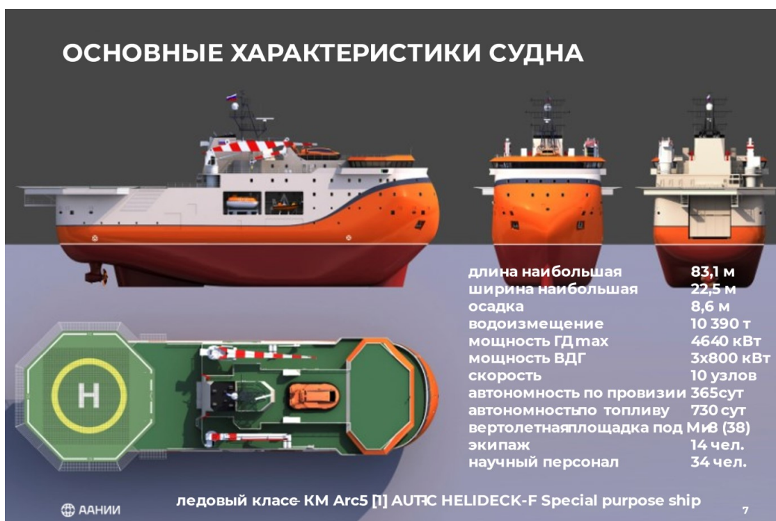
The main characteristics of the North Pole ice-resistant self-propelled platform (AARI archive)
